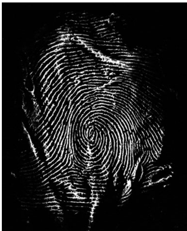
FIG. 3—A negative fingerprint obtained by the latex technique from the mummified forefinger of the left hand.
